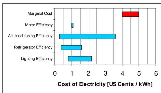
Figure 4.7: Energy Efficiency Cost per kW
