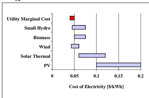
Figure 4.5 summarizes the per-kWh cost of renewable energy technologies that are presented in the previous sections. It can be observed that, by the year 2000, some renewable energy technologies such as wind and small hydro are expected to cost about the same as the utility's marginal cost of electricity in Southeast Asia. Other technologies such as photovoltaics and solar thermal will still be higher than the marginal cost.
