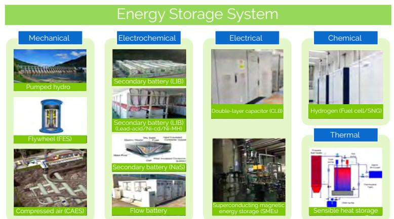
\*Mechanical, electrochemical, chemical, electrical, or thermal.
