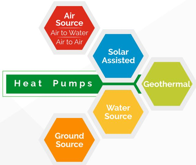
An air source heat pump (ASHP) takes low grade heat from the air, and boosts it to high grade that can be used for domestic heating or any other purpose. The pump uses less electricity than the heat it produces. The performance of an ASHP is similar to a refrigerator, but works in a reverse mode. ASHPs find applications in domestic space heating and hot water supply.
