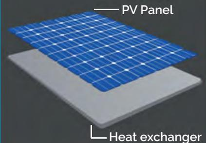
PV panel generates electricity and in addition, transfers heat to heat exchanger
